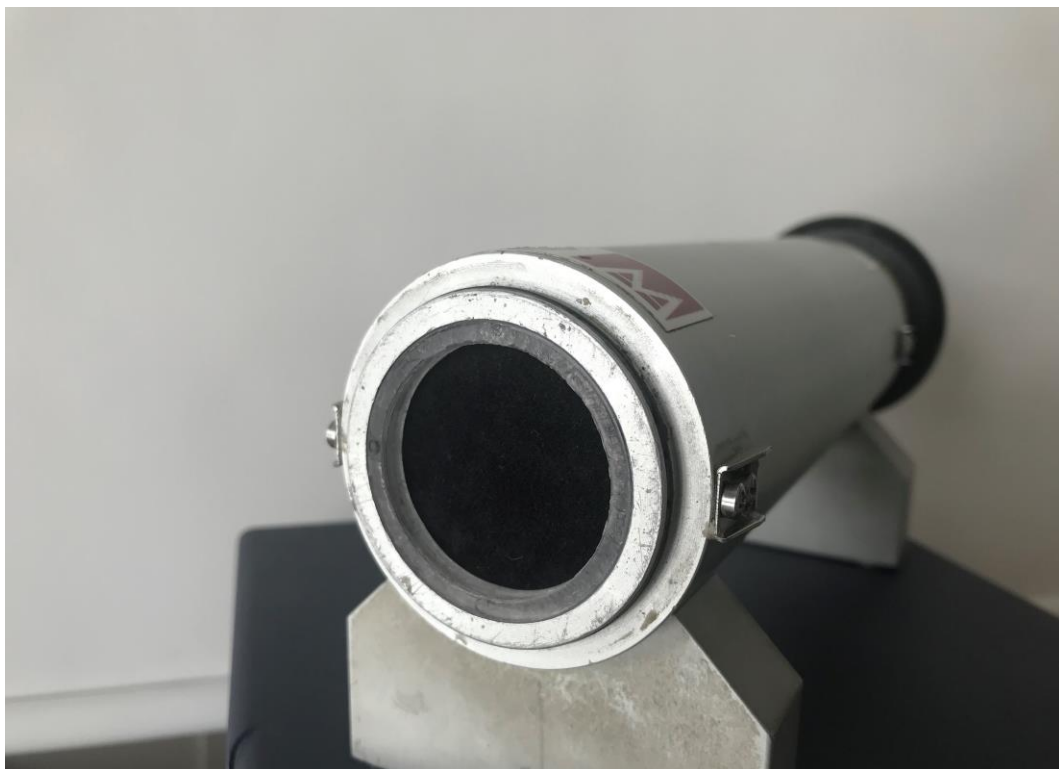
Figure 2 – Sample of panel covered with the fabric inside the measurement tube
