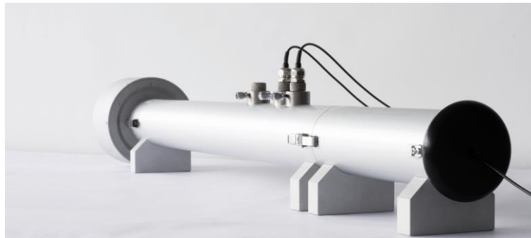
Figure 3 – Acoustic impedance measurement tube
